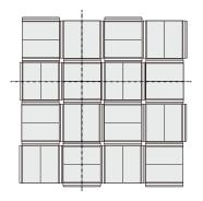
When doing layout Butterfly at checkered pattern, please place pieces along with the center line of the V-shape part for both vertical and horizontal directions. With this layout, the top V-shape parts connected and positioned on the same line. There will be a small opening square at the center of 4 pieces with about 10mm square. The edge lines on the wall will not be straight.
